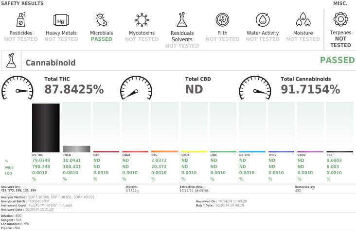
Full spectrum cannabinoid analysis utilizing High Performance Liquid Chromatography with Photo Diode Array detector (HPLC-PDA) for analysis. (Methods: SOP.T.30.500 for sample homogenization, SOP.T.30.031 for sample prep, SOP.T.40.031 for analysis on Shimadzu LC-20X0 series HPLCs). Potency results for cannabis flower products are reported on an "as received" basis, without moisture correction.
